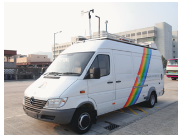
“大氣監測走航平台”可即時搜集本港空氣質量的數據。 The new “Mobile Real-time Air Monitoring Platform” collects air quality information in real time.
