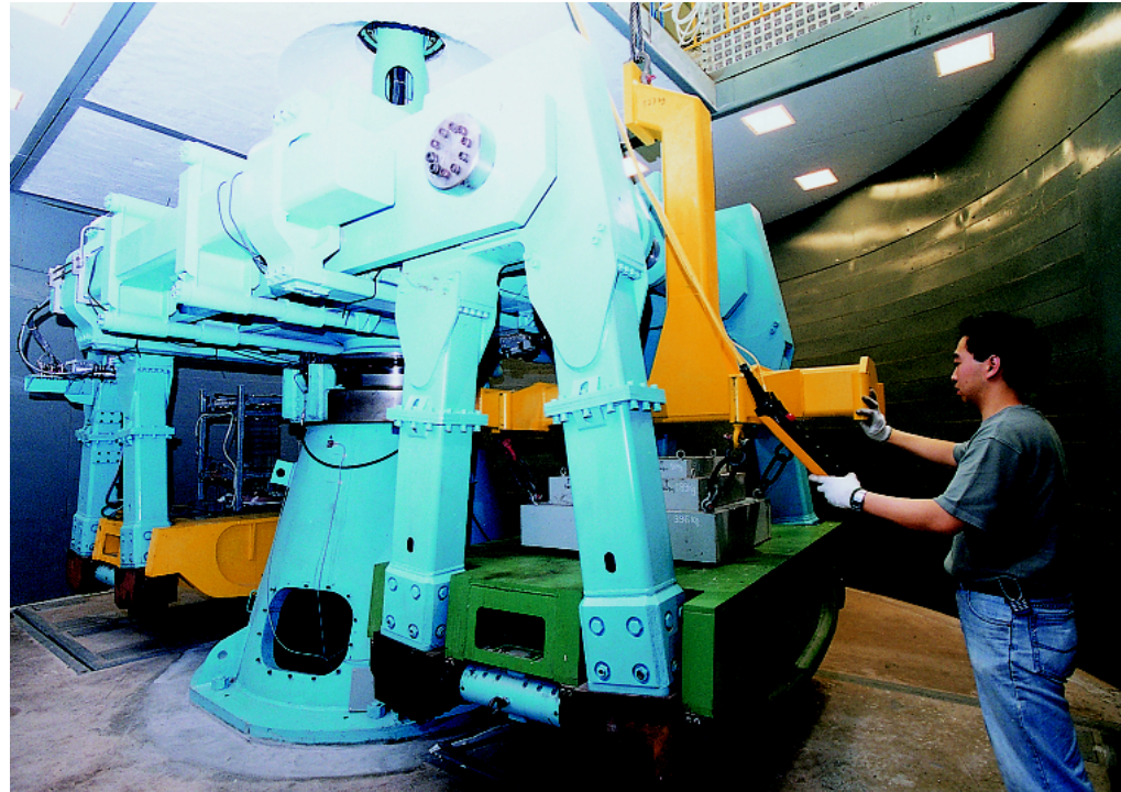
科大岩土工程離心機實驗所配置了最先進的岩土工程模擬設施，改進不同工程項目的設計、素質、安全及技術。 The Geotechnical Centrifuge Facility is equipped with cutting-edge geotechnical modeling facilities to enhance the design, quality, and safety of engineering projects.
